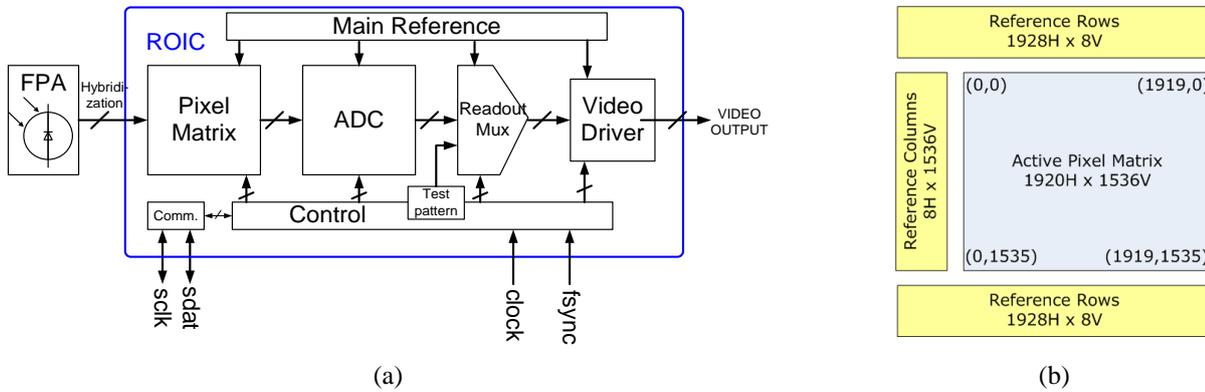
**Fig. 2** (a) ROIC functional block diagram. (b) A scheme of the pixel matrix structure
