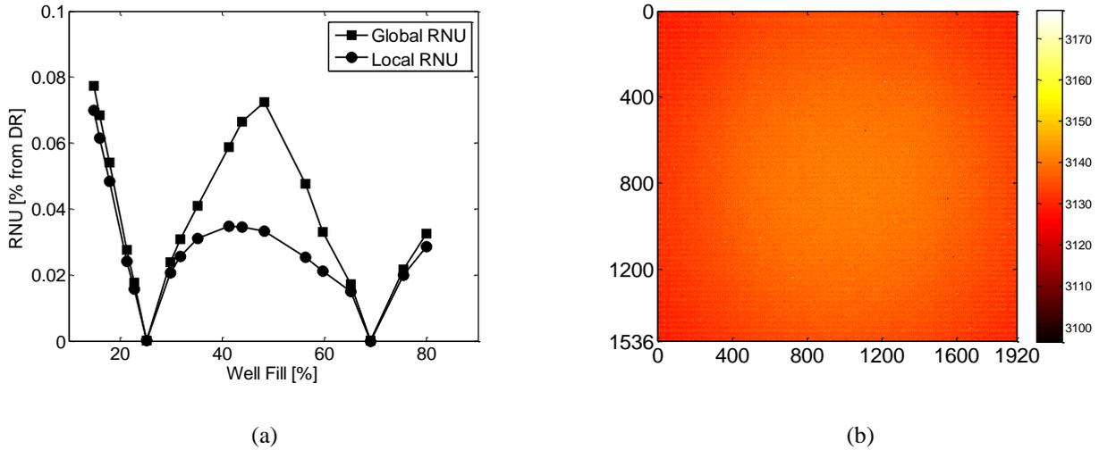
**Fig. 4** (a) RNU as a function of well-fill at F/4, 77 K. The signal is varied by changing the black-body target temperature at constant integration time. (b) An image of a uniform target at 50% well-fill. The color scale is in digital levels. No Bad Pixel Replacement (BPR) was applied.
