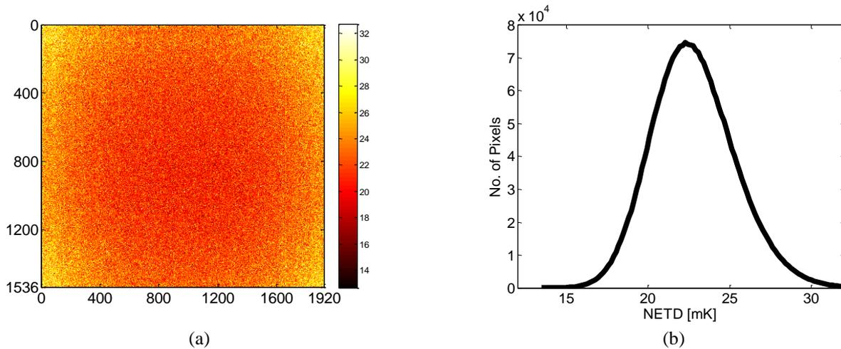
**Fig. 3** (a) NETD image at 50% well-fill, F/4, 77 K. The color scale is in mK. (b) NETD histogram of the data in Fig 3(a). The average NETD is 22.5 mK and the standard deviation is 2.5 mK.
