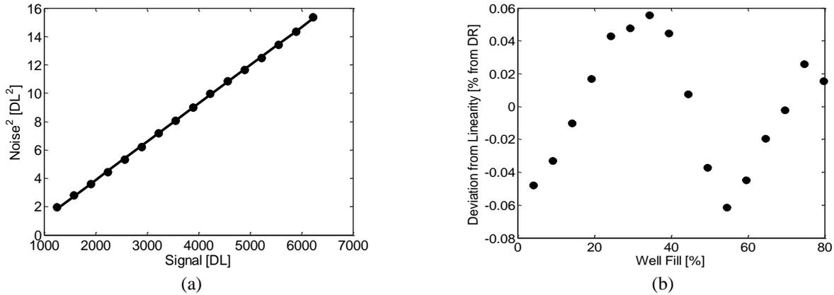
**Fig. 1** (a) Squared noise as a function of signal in digital level measured for the Blackbird InSb FPA, where the integration time is varied (b) Deviation from linearity. The well-fill is varied using the integration time.
