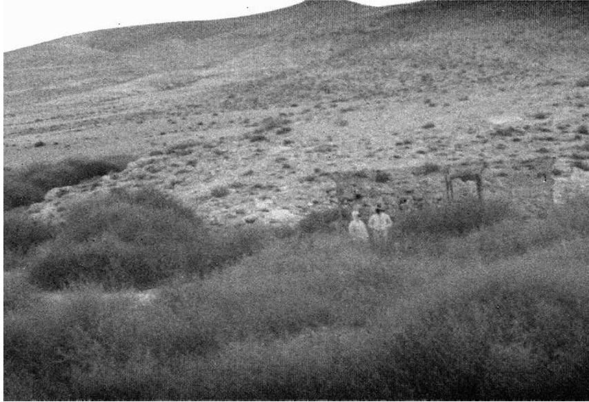
Figure 5: SWIR Image (with Cardinal 640 FPA) captured under starlight conditions (F/1.5, 50mm focal length)
