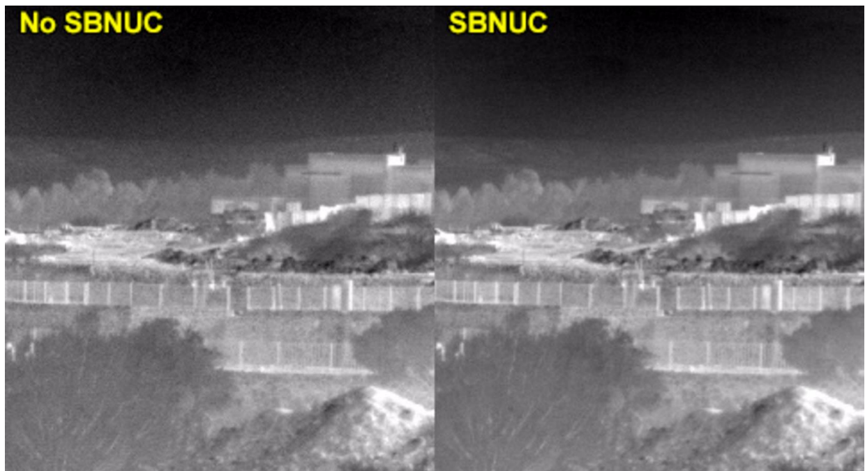
Figure 7 – Scene-based NUC removal of residual fixed-pattern
