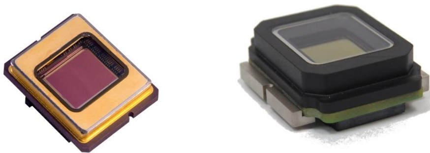
Figure 3: Image of the InGaAs detector in Ceramic package (left) and in "PCB" type package (right)
