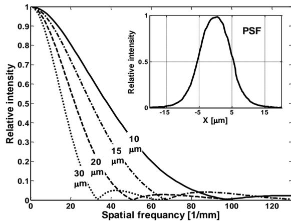
**Figure. 5** MTF curves of InSb FPAs with four different pitches: 30, 20, 15 and  $10\mu\text{m}$ , corresponding to SCDs Blue Fairy, Sebastian, Pelican and Blackbird FPA's, respectively. Insert: Cross section of the PSF image (Fig. 4) at  $Y=0$ .
