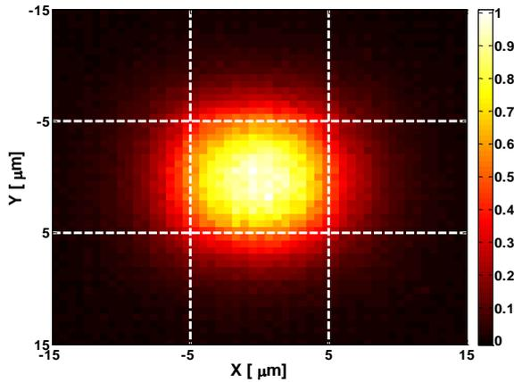
**Figure. 4** PSF image of InSb  $10\mu\text{m}$  pitch, the pixel borders are indicated by white dashed lines.
