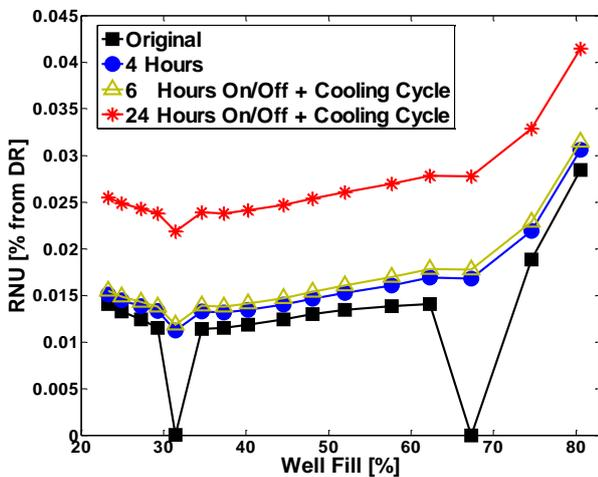
**Figure. 9** RNU at F/3 as a function of well-fill measured at different times but corrected with the same initial table of NUC coefficients.
