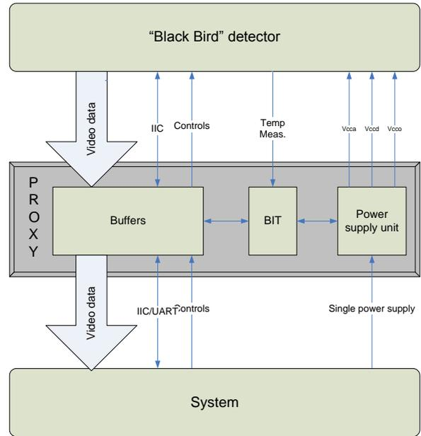
**Figure. 10** Scheme of the proximity electronics.
