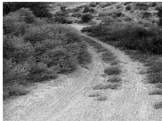
Figure 1: SWIR Imager night mode, during 10 km/h drive at complete darkness, illumination < 5 mLux @ F/1.2 optics.
