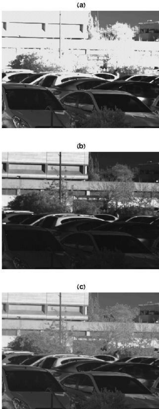
Figure 8: HDR process example: (a) long integration time image; (b) short integration time image; (c) the resulting HDR image
