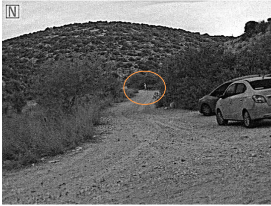
Figure 2: SWIR Imager night mode at moonless night, illumination < 8 mLux @ F/1.2. Person waving detected at a distance of 140 m.
