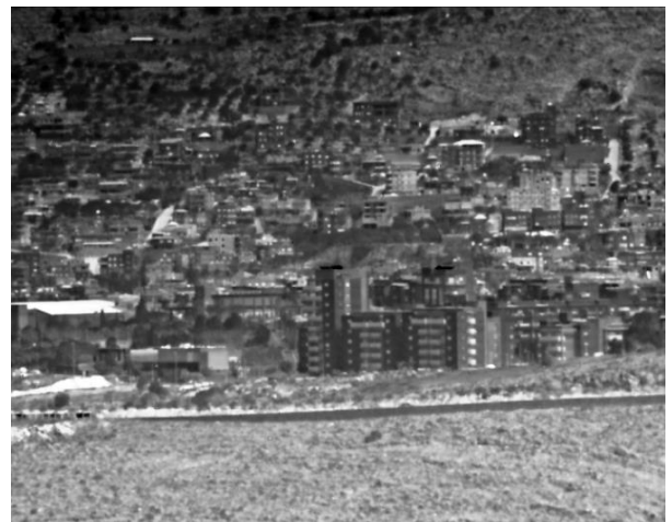
Figure 10. Image registered with the 15μm pitch, 640 × 512 Pelican-D LW FPA operating with F/2.7 optics at 77K (Scene distance = 5 Km)
