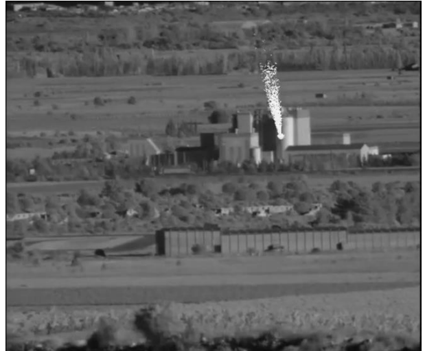
Figure 10: Similar to Figure 9, at a different scenery, the laser pulse from above was detected on the silo
