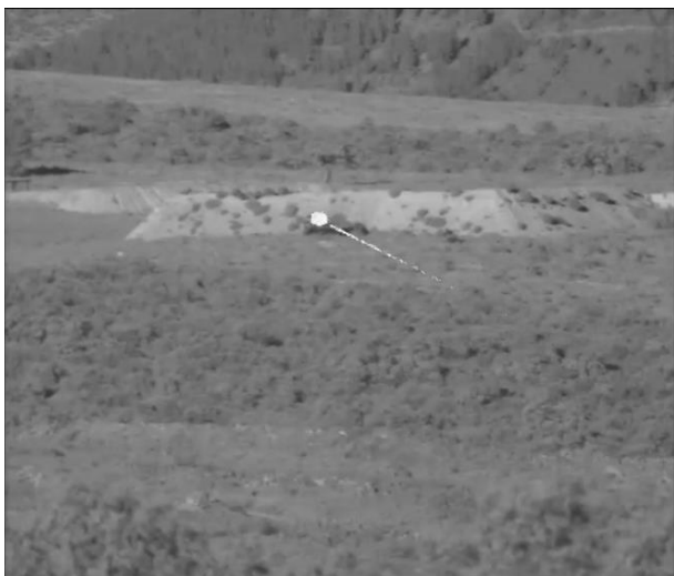
Figure 9: Demonstration of the ALPD mode in Cardinal-1280 . The white spot on the target presents the additional LPD bit in the pixels where a laser pulse was detected. Part of the laser path from right to the target was also detected and is seen on the image as dotted white line
