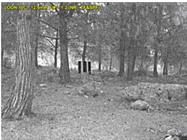
Figure 2: Bar target imaged by the Cardinal-640-LN sensor and F/1.2 optics at Low Light Level conditions
