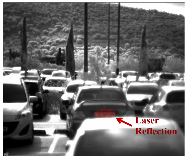
Fig. 3. SWIR Image from an InGaAs sensor with simultaneous laser detection, the laser spot is reflected at the license number of the parked car
